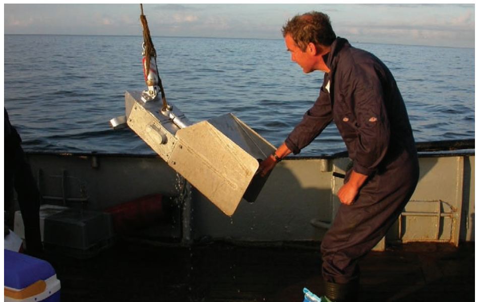
*The team deploys the Continuous Plankton Recorder (CPR) sampling equipment in the North Sea.
