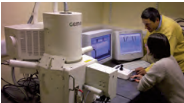
An electron microscope is used to fabricate photonic crystal devices for the study of "slow light" and also applications in optical communications.
