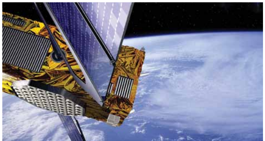
Positioning satellites make use of phased array techniques to modify the beam pattern of their antenna systems. Current research at the University of Bath examines the impact of atmospheric effects on GPS precision and availability.
