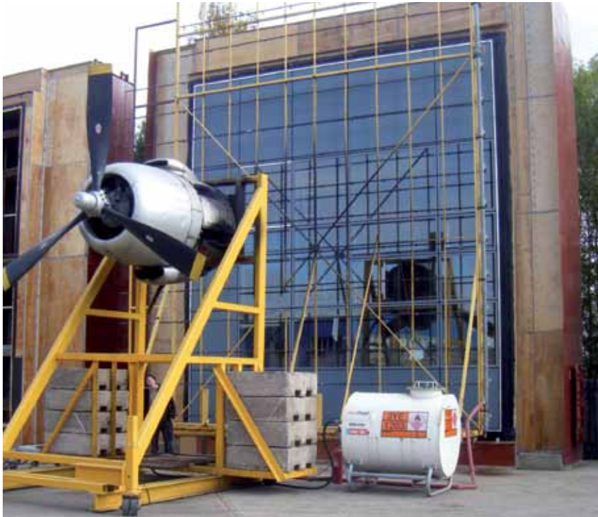
Curtain wall panel being prepared for the aero-engine dynamic water test at Octatube, the Netherlands. The test procedures have been developed by the CWCT centre at Bath.
