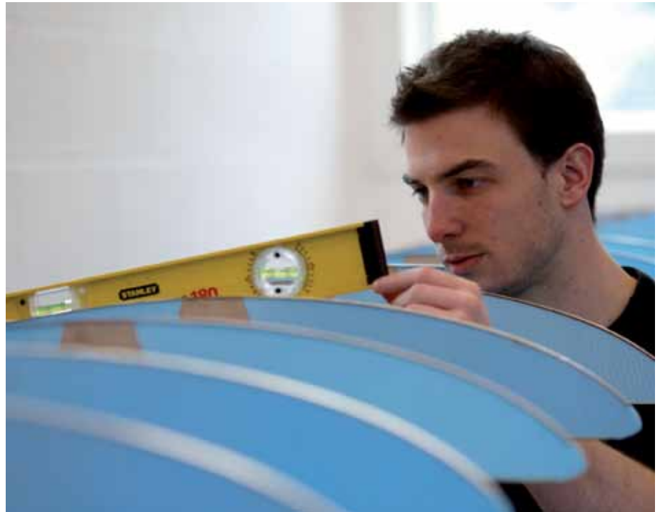
Student checks and fixes the wing ribs to the wing spar for their human powered aircraft.
