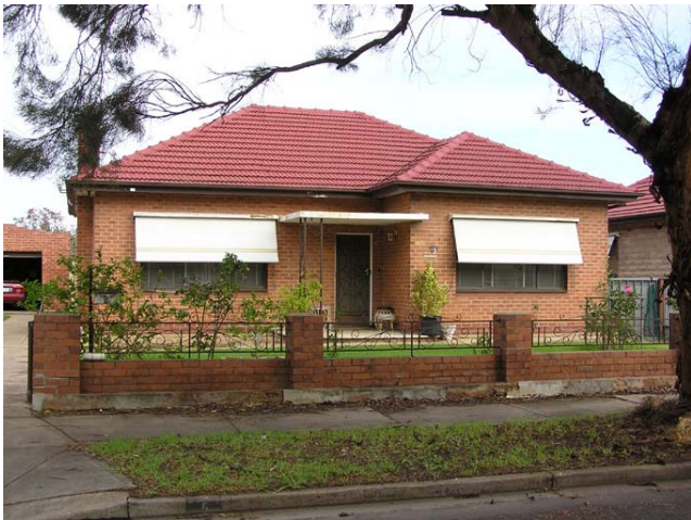
Austerity 1941-1955 - due to World War II, building restrictions limited housing to areas of only 110m 2 , which promoted simpler designs. These homes usually contain two bedrooms, a sitting room, dining room and kitchen.
