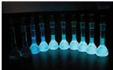
Photoluminescence behavior of metalloles ranging from least polar solvent (left, unaggregated state) to most polar solvent (right, aggregated state).
